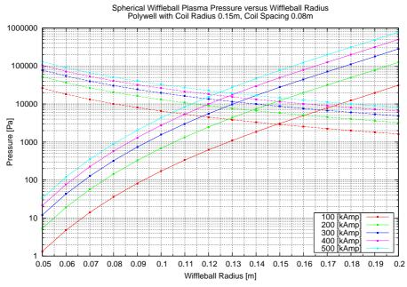
This is for WB6 dimensions and properties. Here the solid line is magnetic pressure, dashed line is the electron kinetic pressure. Where lines of same color cross we have  $\beta = 1$ . This is with  $E_V = 12kV$ .
